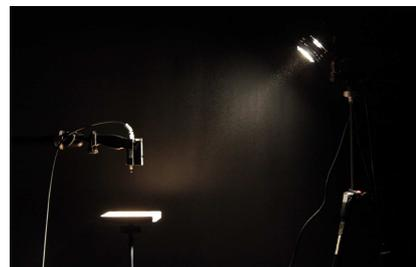
Figure 1. Experimental arrangement: left side the target tray, above the sensor and right side the light source.
