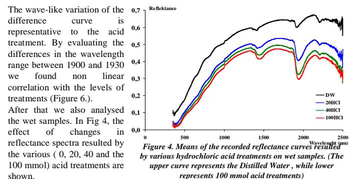
Figure 4. Means of the recorded reflectance curves resulted by various hydrochloric acid treatments on wet samples. (The upper curve represents the Distilled Water, while lower represents 100 mmol acid treatments)
