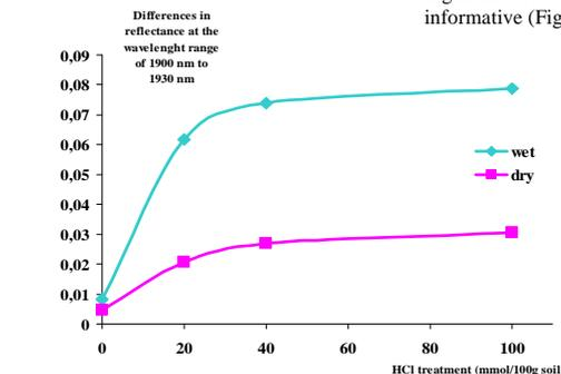
Figure 6. Correlation between the treatments and the reflectance spectra 1900 nm and 1930 nm on dry and wet samples.
