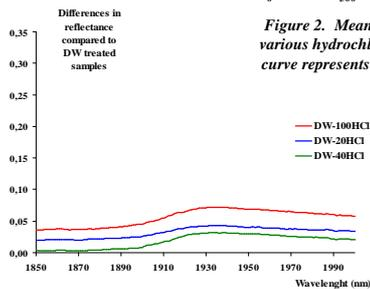
Figure 3. Informative segments of difference spectra regarding the control treatment's spectrum on dry samples.
