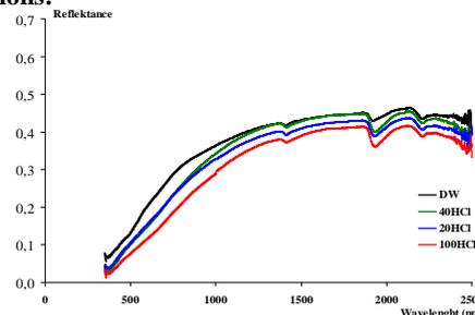
Figure 2. Means of the recorded reflectance curves resulted by various hydrochloric acid treatments on dry samples. (The upper curve represents the Distilled Water, while lower represents 100 mmol acid treatments)
