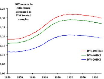
Figure 5. The informative segment of difference spectra regarding the control treatment's spectrum on wet samples.
