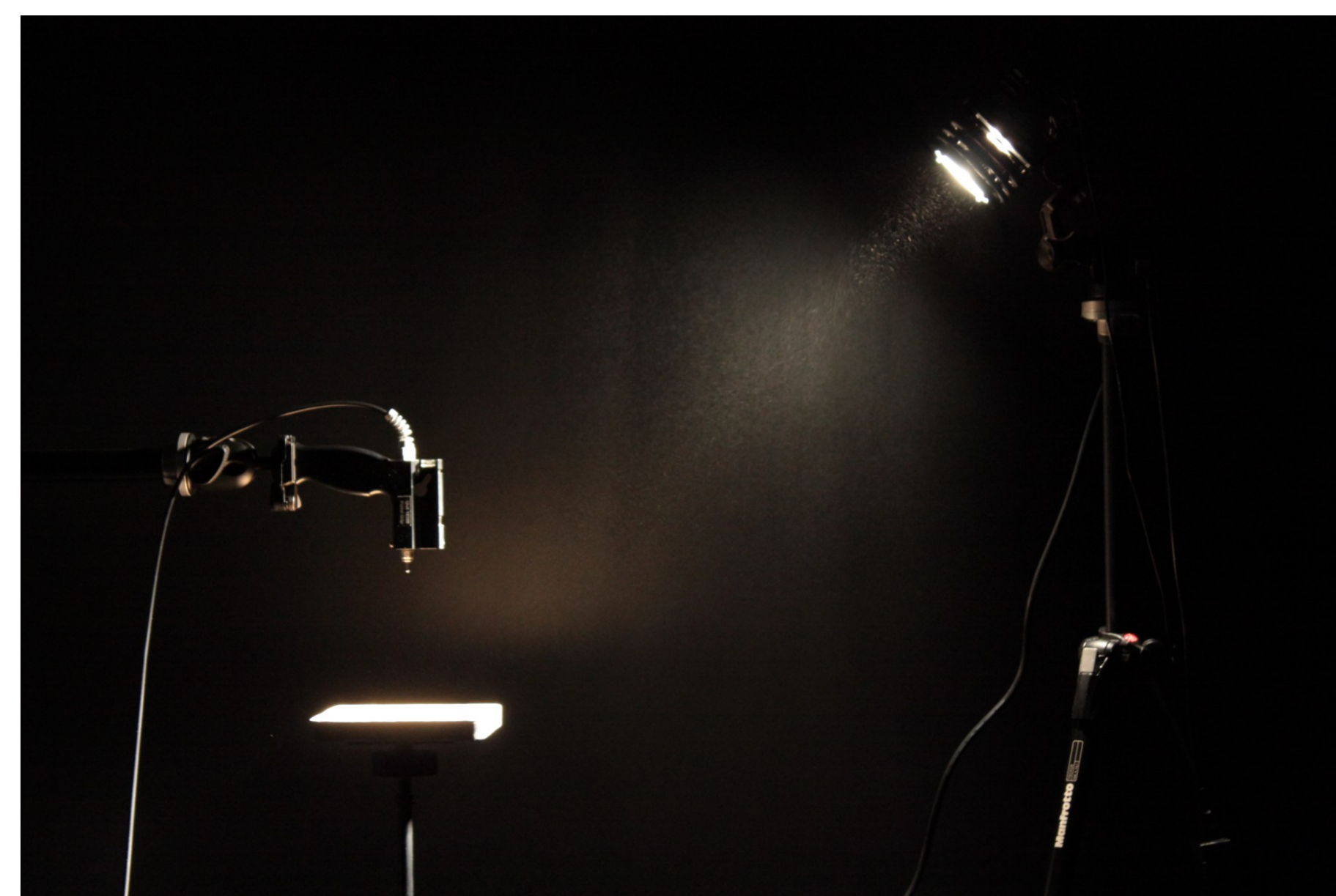
Figure 1. Experimental arrangement: left side the target tray, above the sensor and right side the light source
