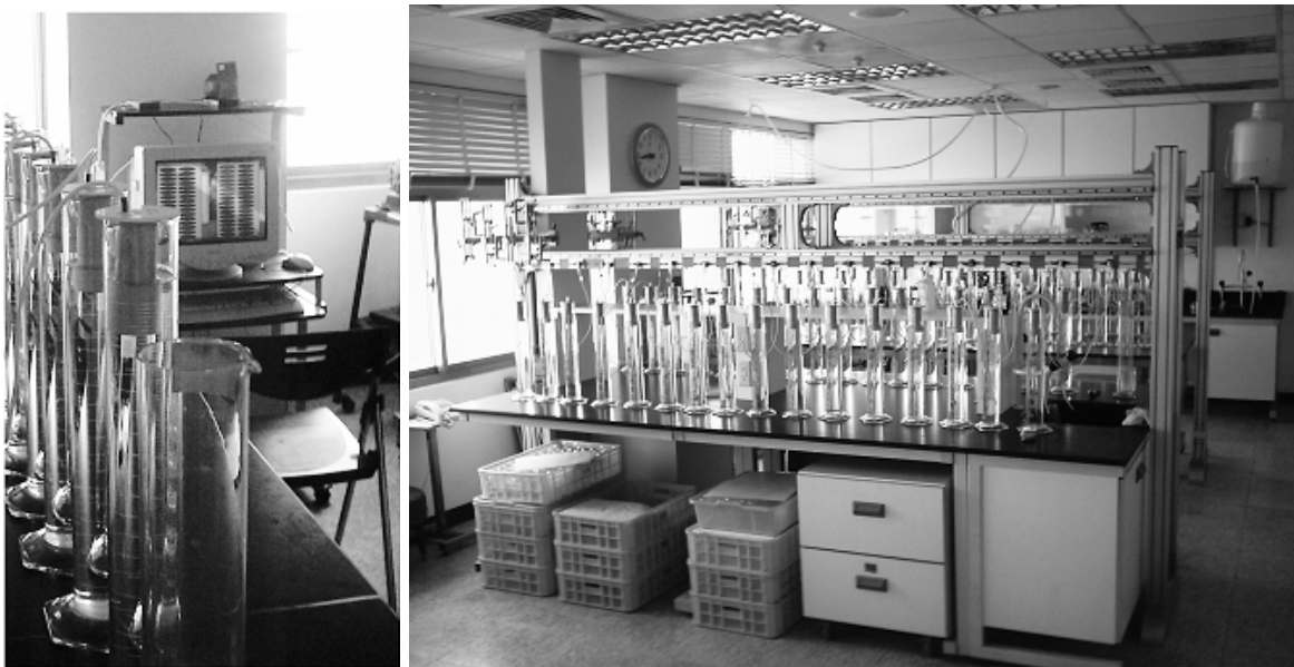
Fig. 10. Laboratory scale pilot-test of parallel 64 cylinder ASTA devices
