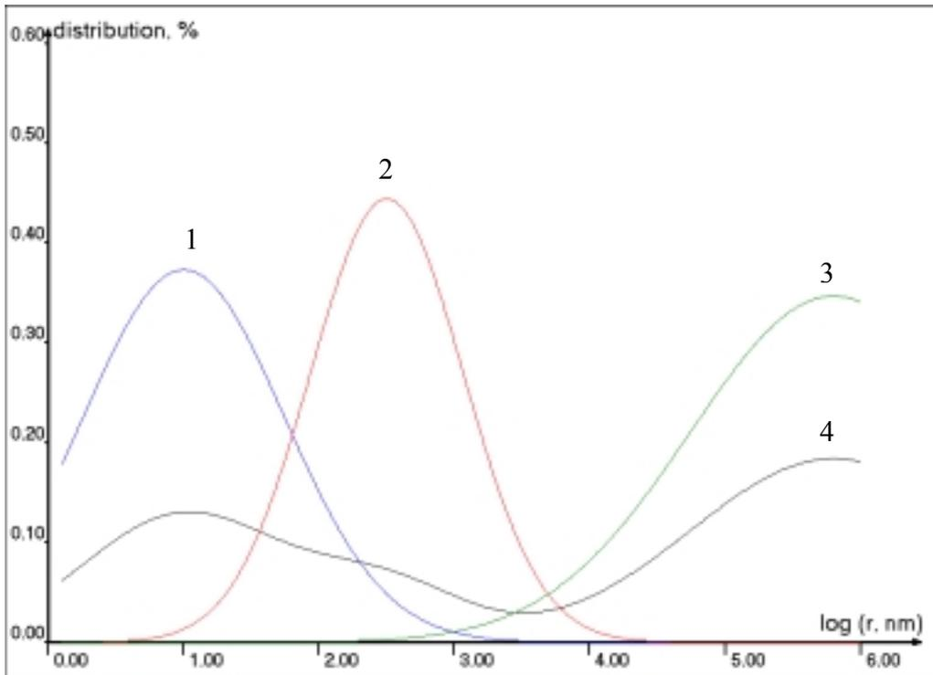
Figure 3. Three extremely different physical soil types (1. clay, 2. silt, 3. sand); and the sum (4.) of the three types normalized for the integral value of the total particle size area
