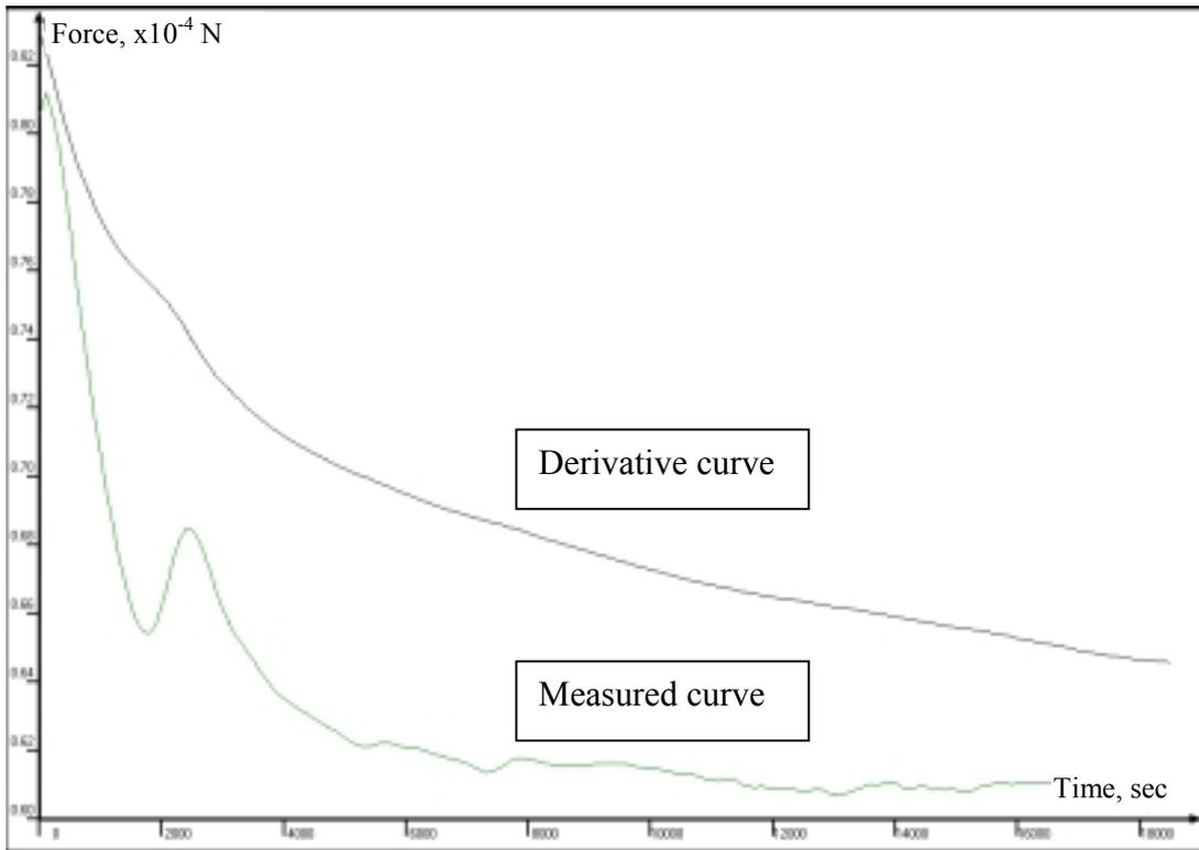
Figure 5. Measured and derived curves from the examination of soil sample GA/1.
