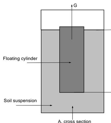
Figure 2. Theoretical outline of the measurement cell
