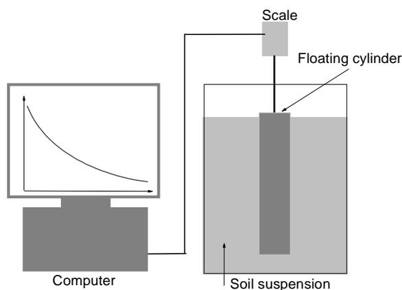
Figure 1. Scheme of the equipment
