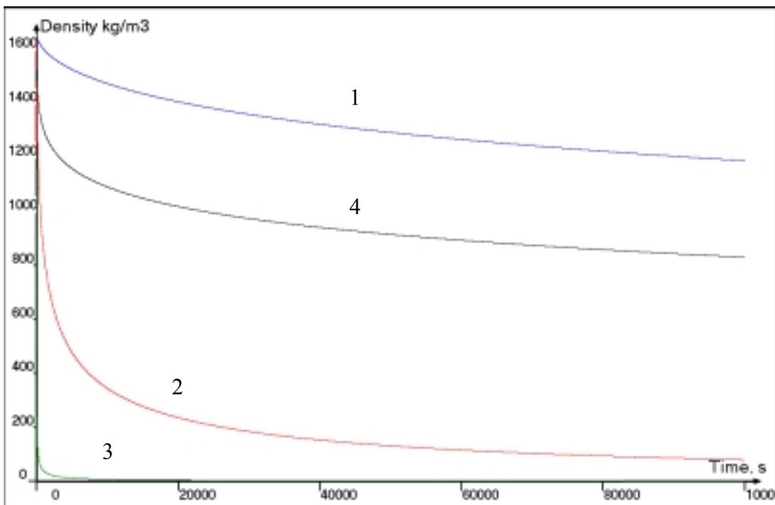
Figure 4. Measurement curves for the same particle-size distributions as seen in Figure 3. (1. clay, 2. silt, 3. sand, 4. sum of the three types)
