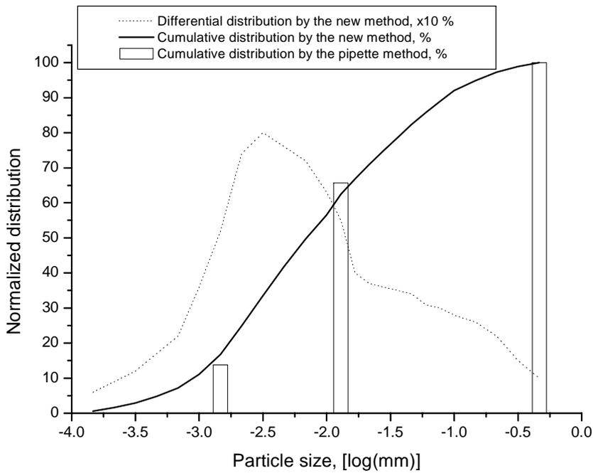
Figure 6. Comparison of measurements using the pipette method and the new automated technique.
