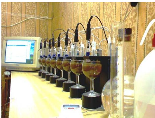
Fig. 1 The multi-channel slow titration equipment
