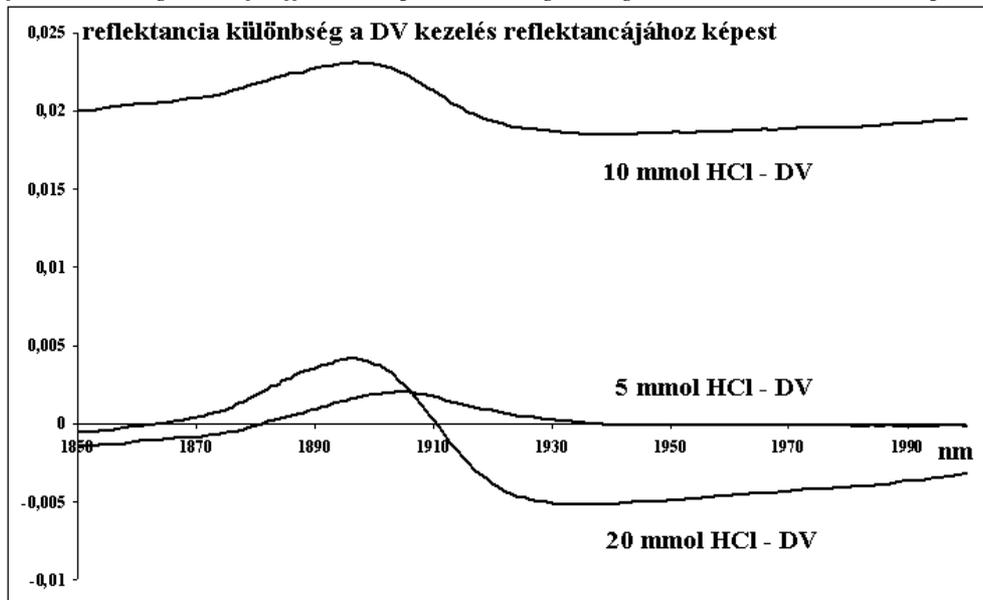
The absolute position of the difference spectrums referred to the x axis not, but the wave-like change is representative to the acid treatment. By evaluating the wavelength between 1900 and 1941, we found significant linear correlation with the levels of treatments (*Figure 5.*)
