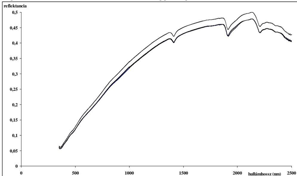
This is proved by the result of the standard deviation between the four acid treatments 0,0093, which is not significantly higher than the one received between the rotated versions 0,0057. The highest reflectance curve was recorded at the treatment of 10 mmol hydrochloric acid, while the others,
