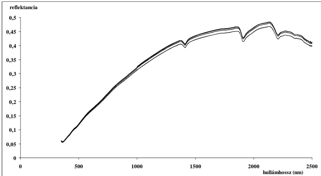
The order of the difference is similar to the changes resulted by the various acid treatments which is presented on the following graph (Figure 3.), where the curves of reflectance are illustrating the 0, 5, 10 and the 20 mmol acid treatment referred to 100g soil sample.
