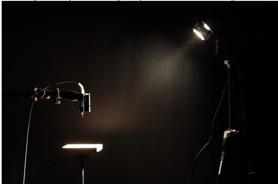
Every sample was measured four times by rotating them with 90 degrees (0, 90, 180, 270). 10 spectrums were recorded (in the whole wavelength of 350-2500 nm) per every measuring, each were composed from 50 scans. The reflectance measurements were calculated from the ratio of reflected light from the certain soil samples and the white reference values.
